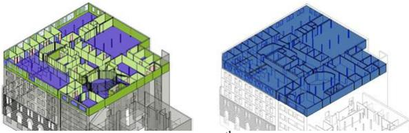
**Figure 6.** Analytical models of 5<sup>th</sup> Floor using gbXML.
