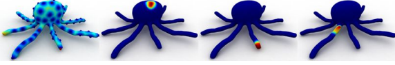
Figure 1: (left) One hundred geodesic farthest point samples on a mesh colored by distance to the closest sample; (right) partition of unity basis functions corresponding to the three red samples.
