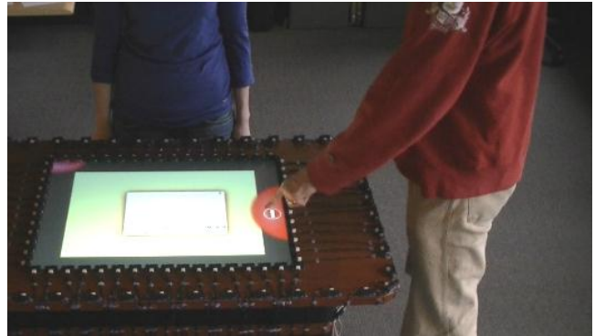
Figure 11: If the tabletop has been placed in the 'Do Not Disturb' mode, all logged out and potential users will be greeted with a 'prohibited' glowing red orb, encouraging them to walk away from the table and not bother those currently engaging with it.
