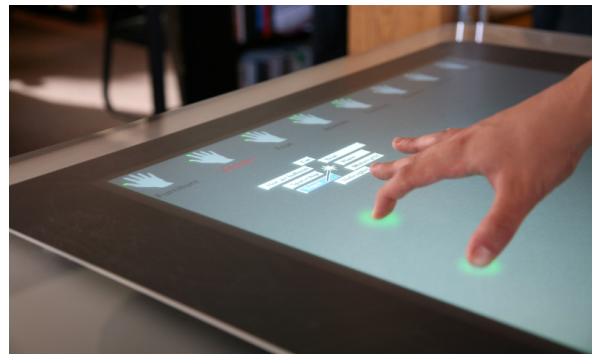
Figure 1. The Multitouch Marking Menu system in use on a Microsoft Surface. The green contact points have been added for illustration purposes.
