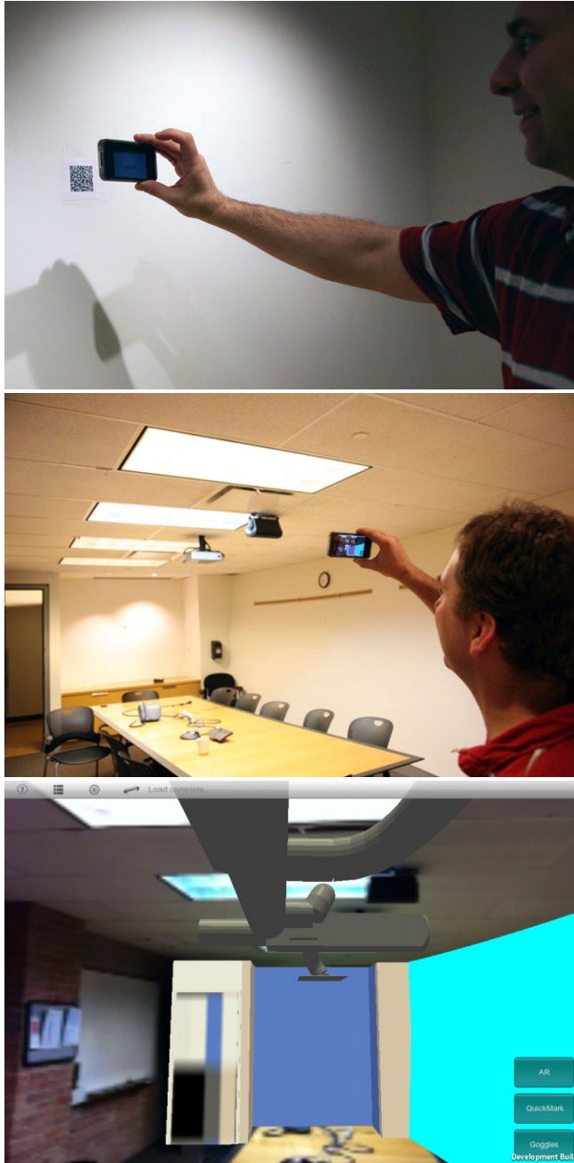
Figure 5. Registering at calibration tag (top). Inspecting HVAC above ceiling (middle). Image shown on mobile device screen (bottom).
