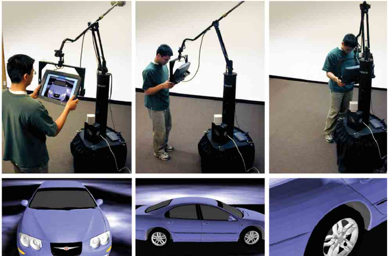
Figure 1. Navigating with the Boom Chameleon. Moving the physical display changes the viewpoint into the virtual world. When the display is moved to the front of the space, the front of the virtual car is viewable; moving to the side shows the corresponding side of the car; and moving closer to the center shows a close-up the car.
